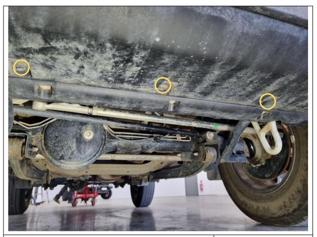
6. Underneath the front, remove 3x 10mm hex screws holding splash guard onto chassis.
