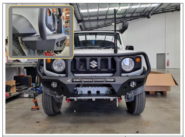
66. With assistance, from another person, align the bar with the edges of the vehicle. The bar should sit symmetric left/right on the vehicle.
