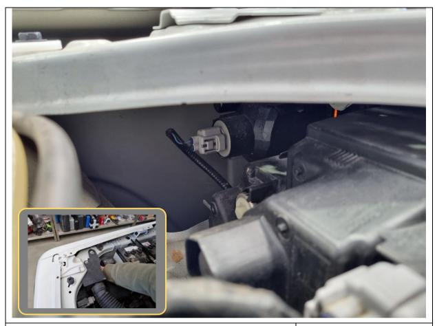
9. Reach in behind the grille and disconnect the indicators, 1x connector per side.
