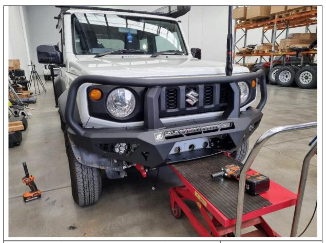
62. Using a lifting trolley, trolley jack or mate lift the bar onto the mounts and secure with M10x30 hex bolts, heavy duty flat washers, flange nuts and Nyloc nuts. Leave finger tight at this stage.
