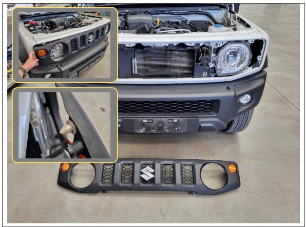
10. Starting from the outer end, gently pull the grille outwards and unclip it from the vehicle.
