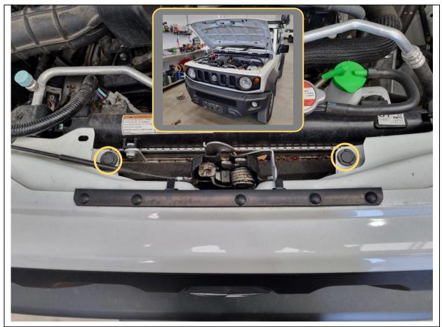
7. With bonnet open remove 2x clips holding grille onto the body.
