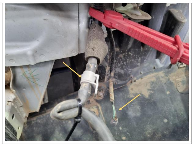
15. Unplug fog light wiring loom on both sides and disconnect headlight washer on LH passenger side.
