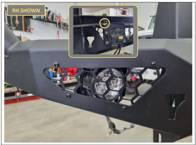
51. Fit the light mesh panel with lights to the inside of the bull bar wing and secure with 4x M6x16 black button head bolts, black washers and flange nuts.
