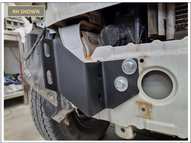
29. Loosely fit the inner chassis bracket as shown, with 2x M10x30 hex bolts, heavy duty washers and flange nuts fed through inside chassis through the large hole. Do this for both sides.
