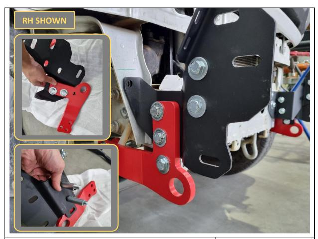
39. Fit the outer chassis bracket with the same bolts and crush tubes as before, but this time with the tow point sandwiched on the outside, as shown.
