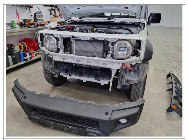
16. Fully remove the bumper and set aside.
